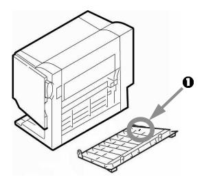
4. Hold the clear band perpendicular to the cover and slip one end over the tab (1), then pivot the band 90 degrees (2) so that it is aimed toward the finisher:
